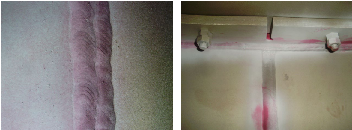
Figure 4-2 Appearances of lining welds of DP28W™
