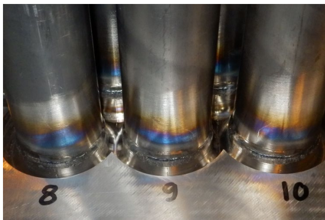
Figure 3-1 Appearance of IBW with DP28W™
