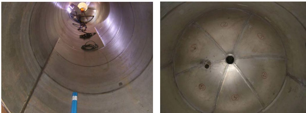
Figure 4-4 New Reactor lined with DP28W™
