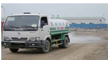
Water sprinkling truck
